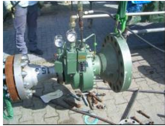
b) Regulator with sound damper
