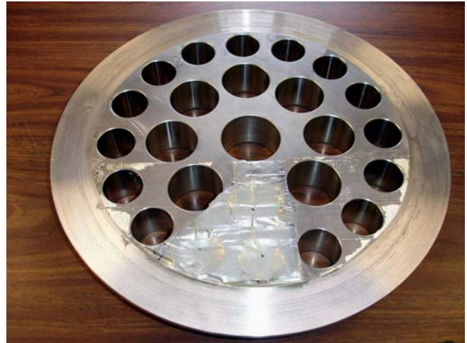
Figure 22 – 3 Holes Blocked Flow Conditioner
