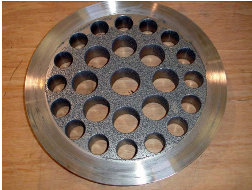
Figure 19: 12-inch CPA with “Texture Paint”
