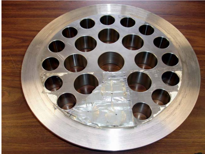
Figure 9: 12-inch CPA with 3 Holes Blocked
