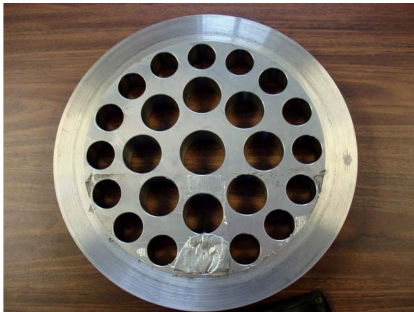
Figure 12: 12-inch CPA with 1 Hole Blocked
